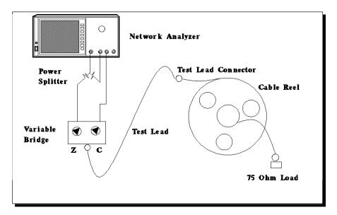
Figure 2. SRL test system setup with variable bridge
