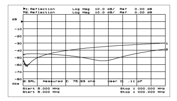
Figure 5. 1000 meter cable with connector mismatch.
