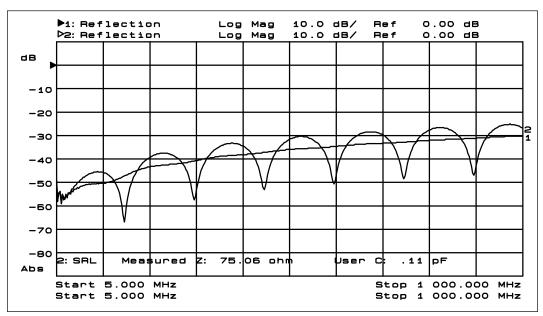
Figure 6. 1000 meter cable with mismatch at 1 meter
