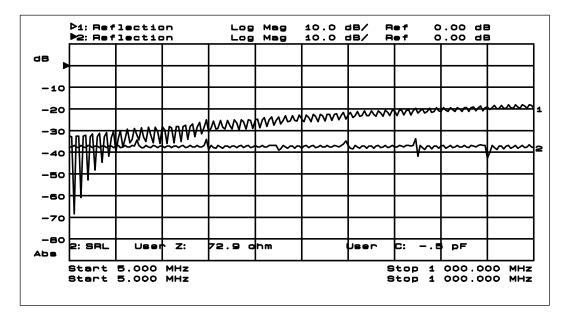
Figure 4. 500 meter cable SRL with fixed bridge and connector compensation
