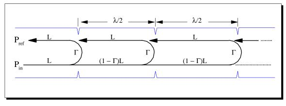
Figure 1. Periodic bumps in a cable
